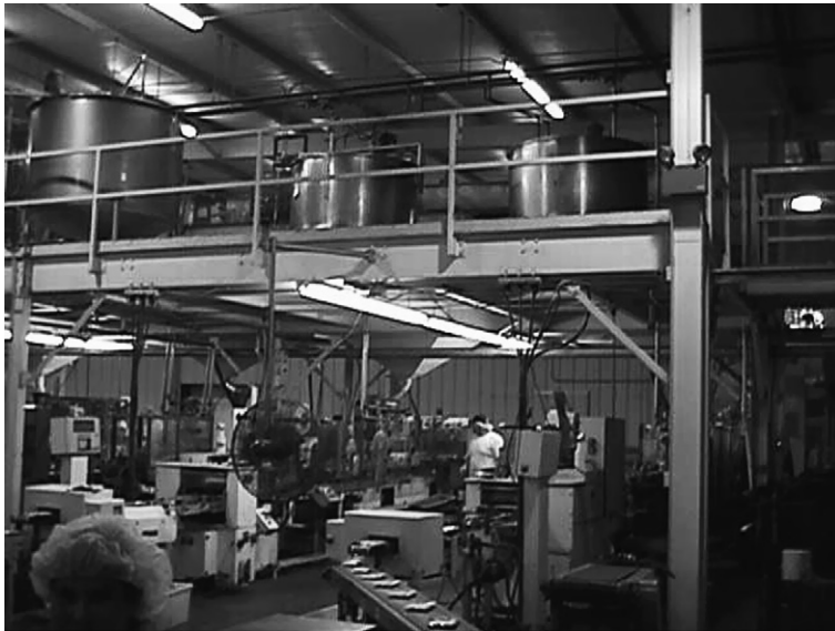
FIGURE 3.1 Sentinel microwave popcorn plant with holding tanks in the mezzanine above microwave popcorn packaging line.
